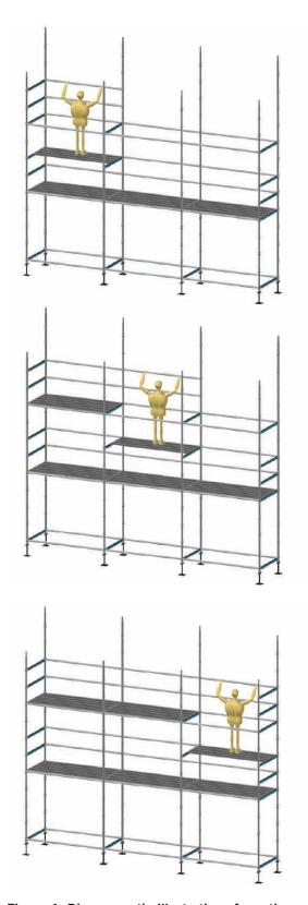
Figure 4: Diagrammatic illustration of erection and dismantling using platform option for a five plank wide scaffold. Note: scaffold is shown against an existing building, so guardrails only needed on external face. Toeboards and lower mid-rails omitted for clarity.
